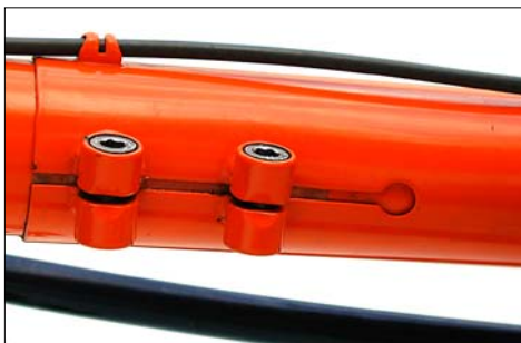
The rear end of the front boom must never be visible in the clamping slot.
