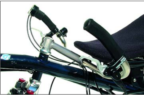
The handlebars are connected to the front fork with an A-Head stem. The two bolts on the side of the stem clamp it to the steerer tube of the front fork.
