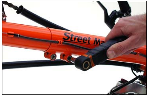
Unscrew the clamping screw to adjust the front boom.
