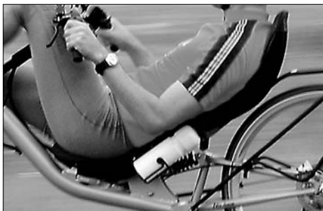
An ideal position for water bottle cages is at the side of the seat.
